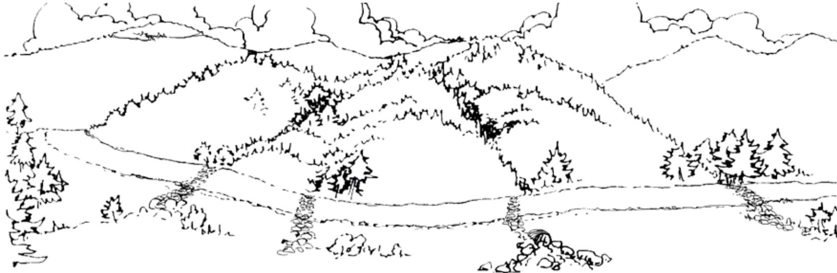
Provide frequent ditch relief with x-drains or rolling dips. Place outlets in natural drainages if possible. Road building or other construction near a stream, river or estuary can create serious fish habitat damage if the work is not done properly.
